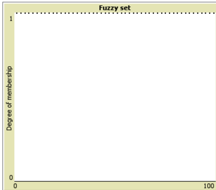
Fig. 15. Membership function of a fuzzy set created running the code: fuzzy:plot fuzzy:interval-with-points-set list [[0 100] 0] (n-values 50 [list (2 * ? + 1) 1])
